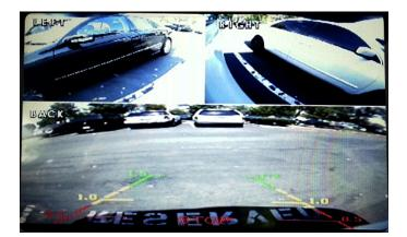
Putting the vehicle in **Reverse** toggles the view of the **BACK**, **LEFT** and **RIGHT** side cameras.
