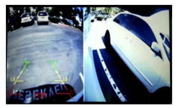
**Right Blinker** toggles the view of the **BACK** and **RIGHT** side cameras.
