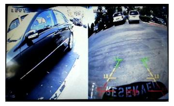
**Left Blinker** toggles the view of the **BACK** and **LEFT** side cameras.
